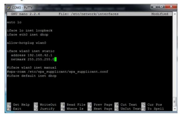
Figure 8- Network configuration for static IP
