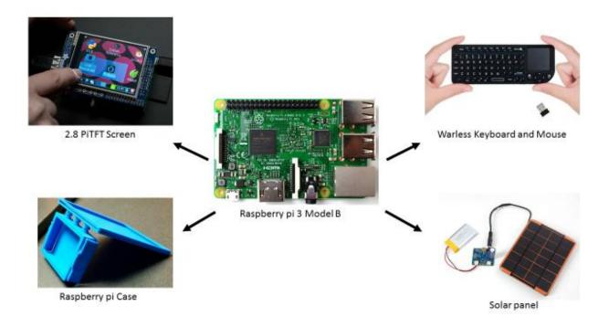
Figure 1: Hardware Design Flowchart
