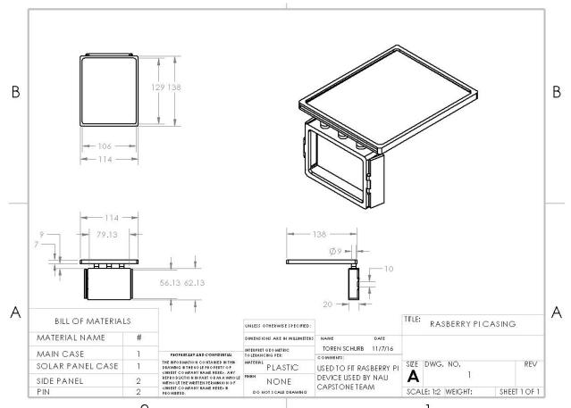
Figure 4: DAGPI Case Dimensions in Solidworks
