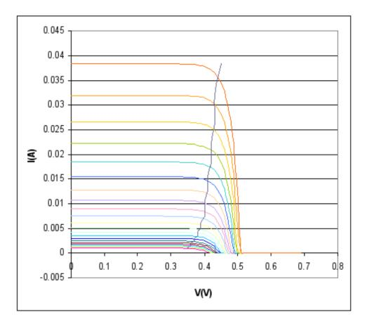
Figure 6: Solar cell I-V curve in varying sunlight
